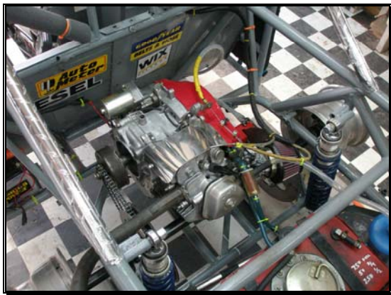
Honda GX390. Note the engine seals...
