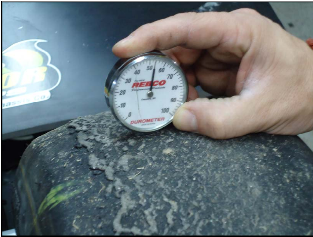
Checking durometer...note the graining across the tire. These run over 130°F depending on track temperature
