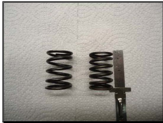
Valve springs; EES 5 coil (left) & MMI 6 coil (right)
